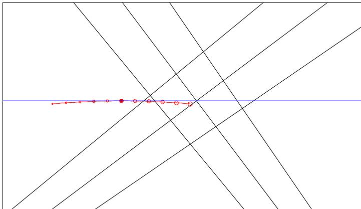
The smallest circle, on the left marks the center of rotation for +5°. The solid circle is 0° and the largest circle on the right is the center of rotation of the boom for -5°. The centers move about 0.009" for each degree of boom motion, covering a range of 0.092" over the ± 5° range. The pairs of intersecting lines are the flexures at the +5°, 0° and -5° positions. Over that range, the intersection of the flexures moves by 0.061".
