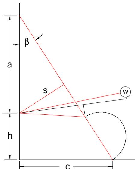
identical. However, differences will appear once the beam moves up or down. In the LaCoste system the *upper* spring attachment is fixed and the line of action of its force will always pass through that point. In the leaf spring system, the *lower* attachment is fixed, and as the beam moves, the intersection of the line of action with the vertical support will move up and down. We should thus expect to see some differences in the behaviors of the two designs due to the differences in geometry.
