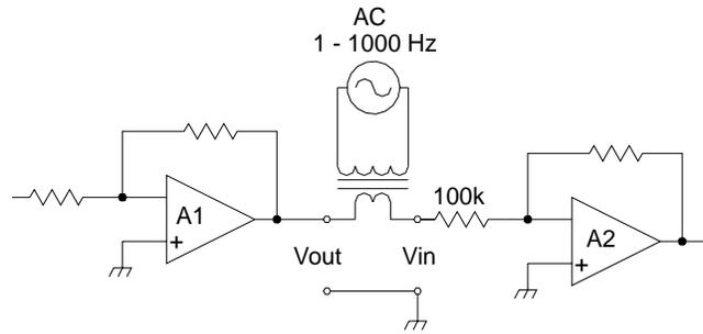
If we assume that the transformer core is approaching saturation at full rated power and minimum rated frequency, an estimate may be made of the secondary voltage available at any other frequency, F. That is  $V_{sec} \leq \sqrt{(P_{max} \times Z_{sec})} \times F / F_{min}$
