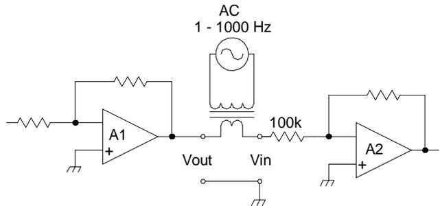
If we assume that the transformer core is approaching saturation at full rated power and minimum rated frequency, an estimate may be made of the secondary voltage available at any other frequency. That is  $V_{sec} \leq \sqrt{(P_{max} \times Z_{sec}) \times F / F_{min}}$
