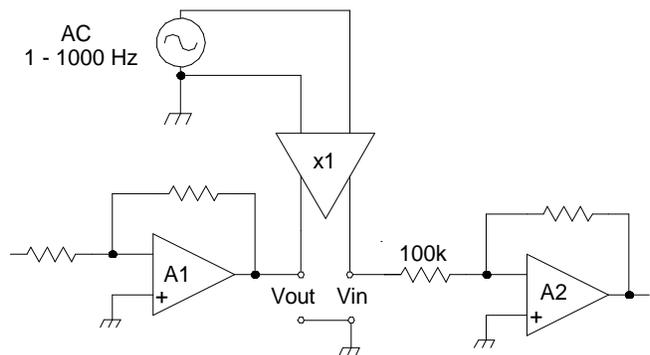
If we are able to insert reasonably high-level signals, an oscilloscope is the ideal measuring tool, preferably one having two traces and good low frequency sensitivity. A blind AC voltmeter will work, but it is still imperative to know that the inserted signal is not saturating the feedback loop, rendering the measurements meaningless, and to also know that you're not just measuring hum or noise voltages. With a scope viewing the two signals, overloading is easy to see, allowing the drive
