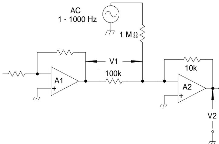
Nonetheless, on occasion, a point may be found which suggests that this kind of measurement could be tried. The circuit we looked at before is a case in point. If we choose to “break” the loop between the 100k resistor and the summing point of A2 we now see the required high impedance upstream and low impedance downstream.
