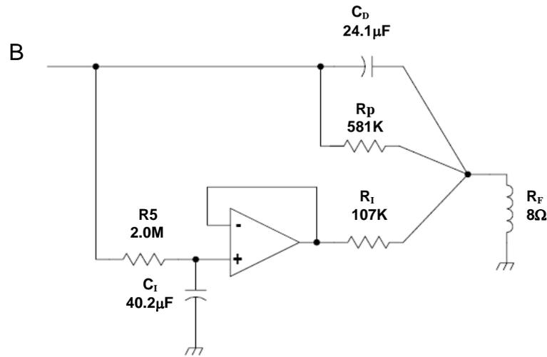
The original circuit had a transfer function from the voltage at 'B' to the current in the feedback coil of:
