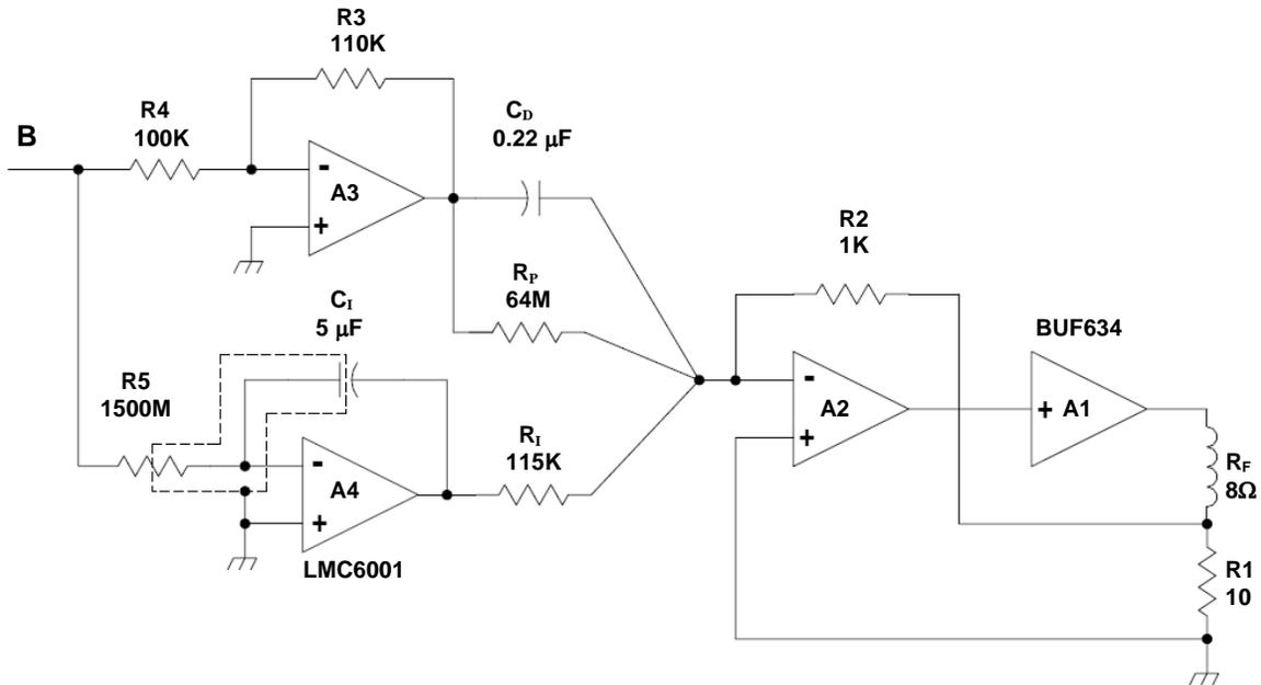
is incorporated into the main feedback loop, which has substantial loop gain at DC, the feedback will simply adjust the mass position by a small amount, sufficient to exactly offset the leakage current, via R5. Nevertheless, because R5 is so large, the input current variations in A4 must be kept quite small to avoid introducing excessive noise in the loop. The LMC6001 has extremely low input current and current noise.
