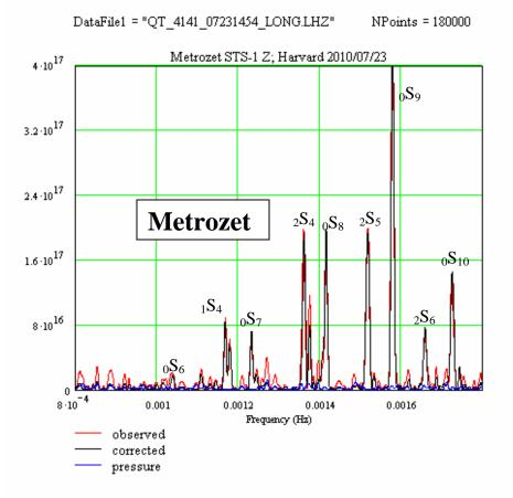
A longer (180,000 second) interval allows Metrozet sensor to observe splitting!
