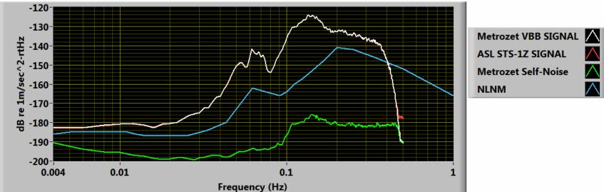
ASL day 274 data: 500 Second Pieces, 80 averages, 0% overlap; equivalent sensor assumption Signal, Incoherent Noise and NLNM PSD
