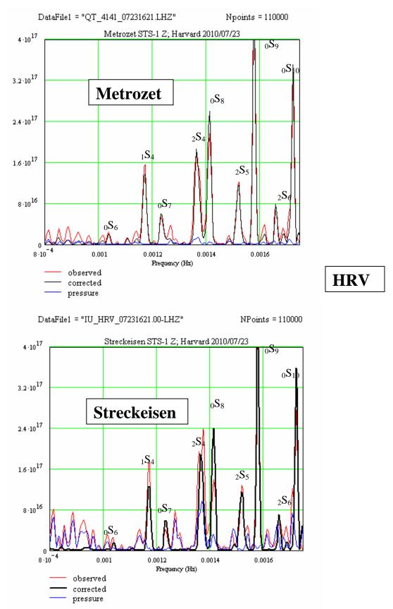
Raw and pressure-corrected spectra from 110,000 seconds of data
