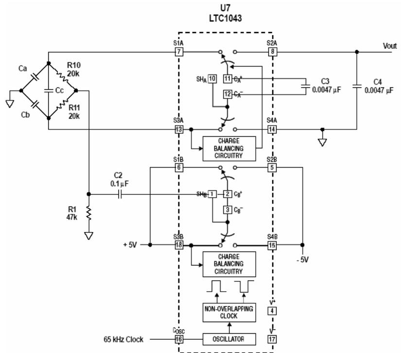
The result is that any unbalanced capacitance creates a voltage across the output capacitor of about 1.3V per mm of sensor motion. The 62.5kHz clock frequency and the capacitor values used, result in a transfer function pole having a time constant of about 0.52ms, representing a frequency roll off at 306 Hz.
