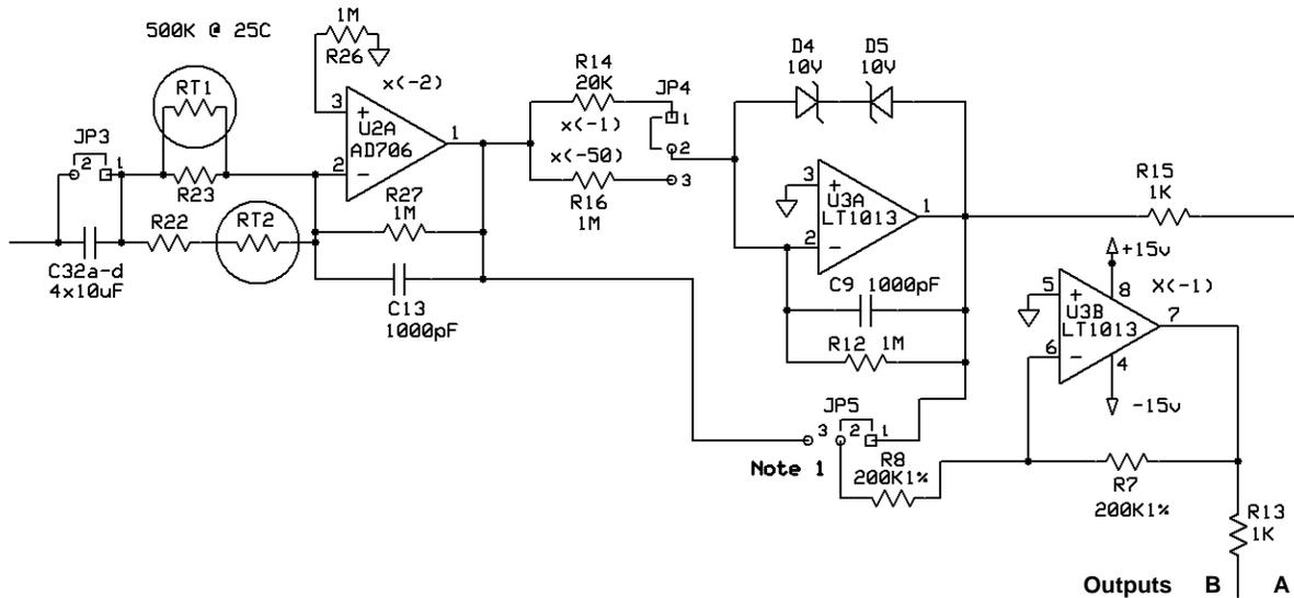
These amplifiers are driven by the output of the feedback loop and are intended to provide flexibility in the choice of output signals and to isolate the feedback loop from the output connections.
