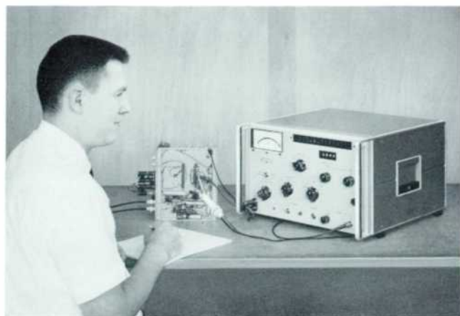
Fig. 1. By using an -hp- AC-21F clip-on probe to couple signal output from -hp- Models 302A or 310A Wave Analyzer into feedback loop, loop gains can be measured easily and without breaking loop.
