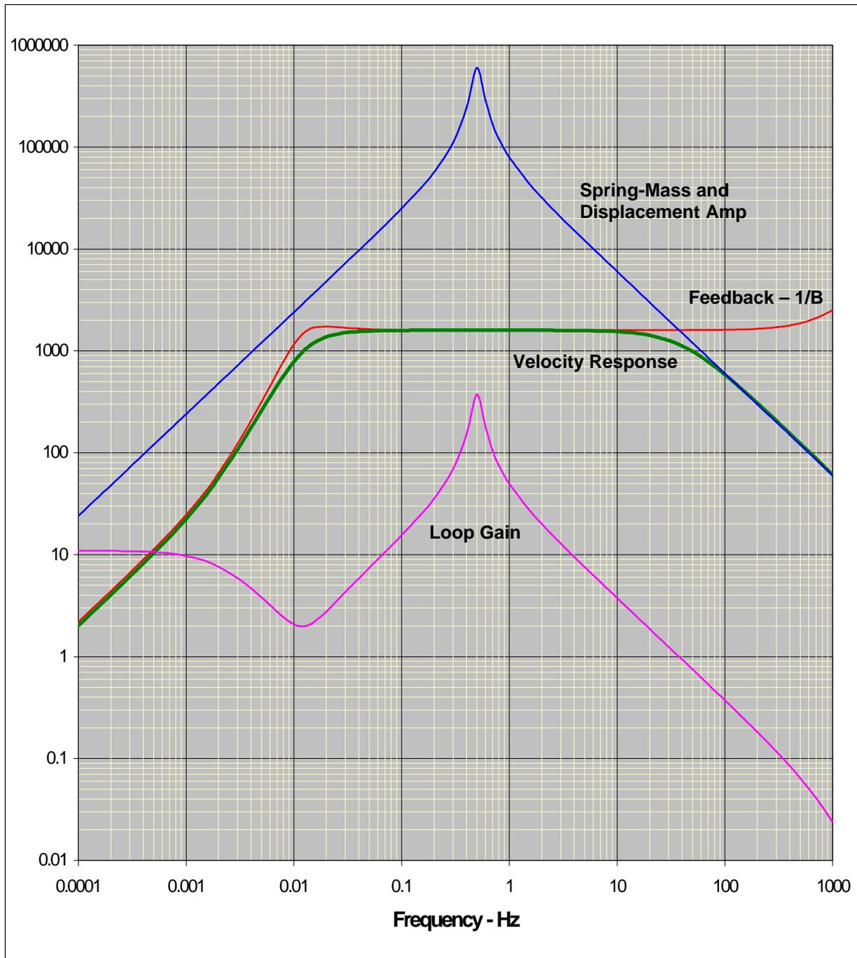
In the loop, with the assumed parameters, it is seen that the loop gain in the 0.01 Hz region gets as low as 2. Because of this, the system response in that region is affected by the spring-mass-amplifier characteristic. To compensate for the additional rounding off of the response function, the feedback path function,  $1/B$  is slightly underdamped.
