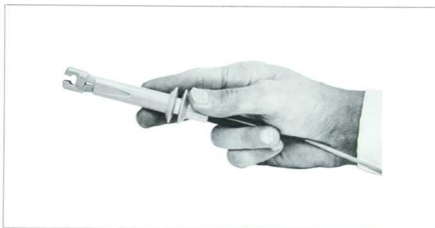
Fig. 3. hp AC-21F clip-on probe, normally used for sampling ac current, is used in loop gain measurements to inject signal from Analyzer into loop.
